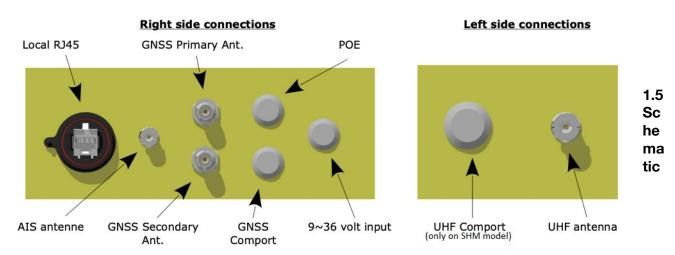
!Always connect the UHF antenna when the unit is powered on!
