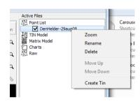
After the data is cleaned up a TIN (Triangulated Irregular Network) can be generated. This can be done by *right clicking* on your XYZ project in the top right and selecting *Create Tin*. A pop up window will appear asking for a name for the new TIN and most importantly a Maximum Edge Length. This maximum Edge Length represents the longest leg of the triangles and should
